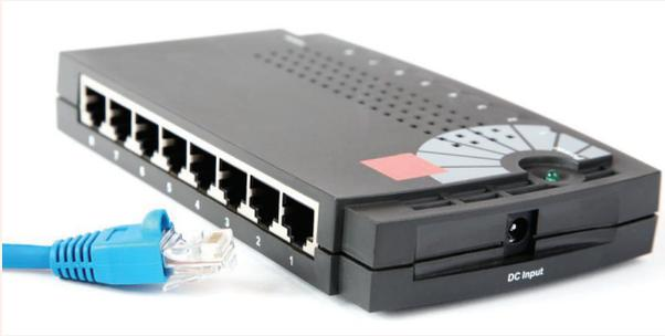
connected to. However, because of its working mechanism, a hub is not so secure and safe. Moreover, copying the data packets on all the interfaces or ports makes it slower and more congested, a fact which led to the use of network switch.
